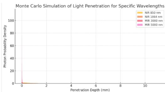
This Monte Carlo Simulation of Light Penetration at Specific Wavelengths. This plot visualizes how NIR (850 nm, 1064 nm) and MIR (3000 nm, 5000 nm) light penetrate biological tissue.
