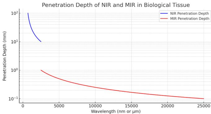
Here is a visualization of the penetration depth of Near-Infrared (NIR) and Mid-Infrared (MIR) light in biological tissue.
